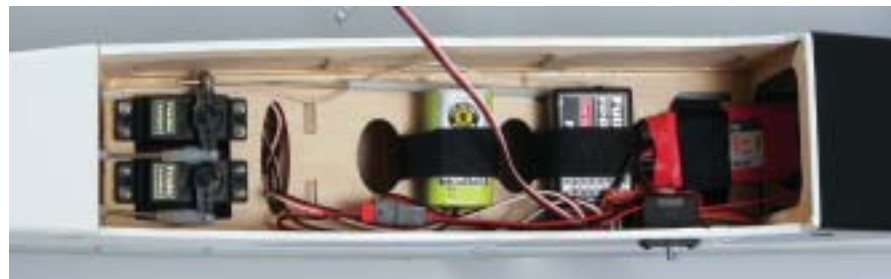
The fuselage features a sturdy plywood subfloor. The radio gear is neatly mounted on top of this floor, while the motor batteries are installed below through a generous hatch.
