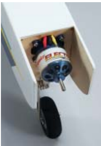
Above: The aileron servo comes pre-installed in the right wing panel, with the pushrod linkages all made up and installed. Join the wings, connect the second clevis to left aileron and you will be ready to fly. Left: The Hobbico ElectriStar C-42 Brushless outrunner offers similar power output to the standard .40 glow engine typically used to fly a trainer of this size and weight.
