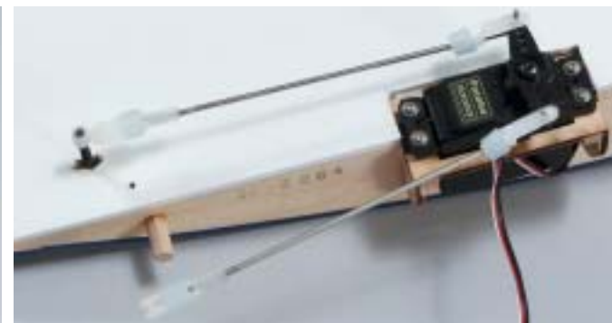
Above: The aileron servo comes pre-installed in the right wing panel, with the pushrod linkages all made up and installed. Join the wings, connect the second clevis to left aileron and you will be ready to fly. Left: The Hobbico ElectriStar C-42 Brushless outrunner offers similar power output to the standard .40 glow engine typically used to fly a trainer of this size and weight.
