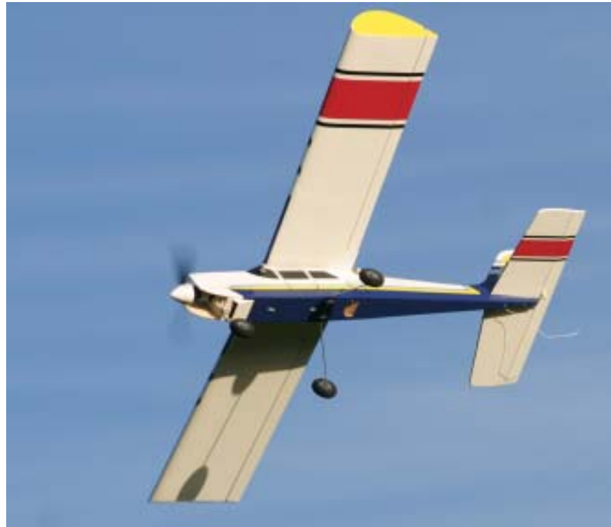
The ElectriStar features bold red bands on the underside of the wing and stabilizer. This asymmetrical color pattern helps orientation during early training when your model would typically be at a higher altitude.
